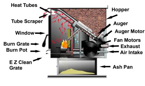
Cutaway View Figure 4
